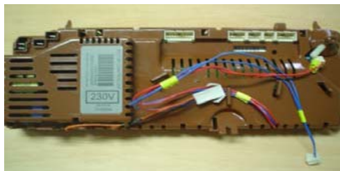
Grey module in brown cases (new) Note: Sticker is grey in colour to help identify module type.
